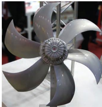
Fig. 1 Fan wheel with curved blades
