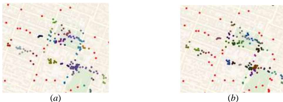
Fig. 6. DBSCAN algorithm: (a) minPts = 3 , \epsilon = 100 ; (b) minPts = 3 , \epsilon = 75
